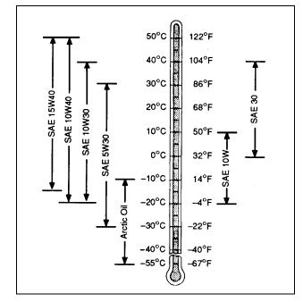
Use oil viscosity based on the expected air temperature range during the period between oil changes.
